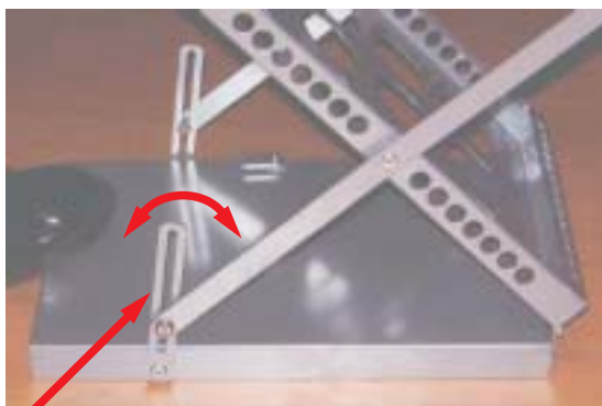
Slider bar Raise unit vertically until slider bar rotates through 180 degrees
