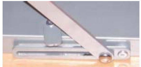
Finally rotate locking tab into place Unit is now assembled Important note : Unit may not be correctly assembled if slider bar is not in the horizontal position
