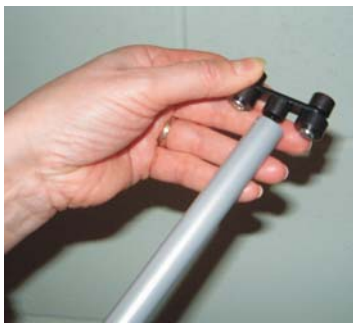
Fit doubler into the top of the bungee pole
